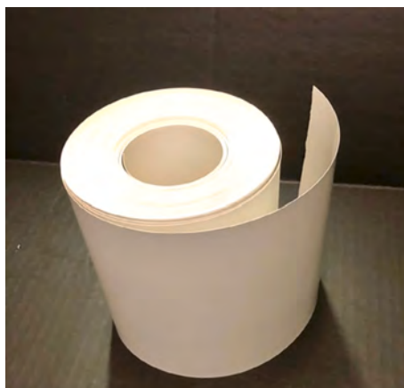
Fig. 39. Photograph of flexible ferroelectric BST/polymer composite tape [198].
